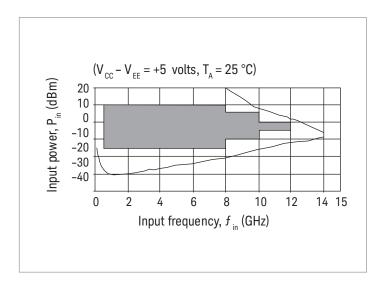
Figure 4. Typical input sensitivity window
