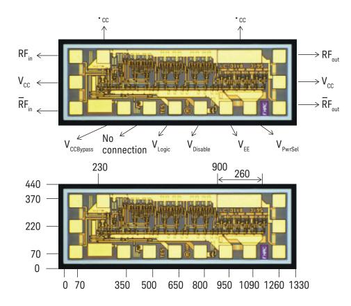
Figure 2. Pad locations and chip dimensions  $% \left( 1\right) =\left( 1\right) \left( 1\right) \left($
