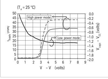
Figure 5. Typical supply current & V<sub>Logic</sub> vs. supply voltage
