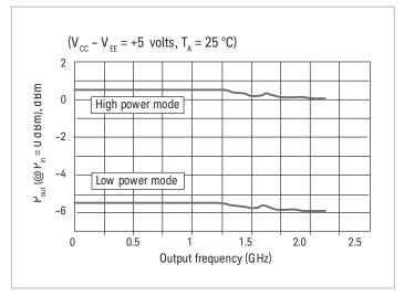
Figure 7. Typical output power vs. output frequency,  $f_{\rm out}$  (GHz)
